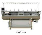
This machine is a global standard for computerized shaping machine with intarsia capability. Even if multiple colors are used, the machine can produce a beautiful pattern with few irregularities. This machine does not pass the yarn to the reverse side, but knits it so that it folds over at the point where the colors switch, minimizing yarn loss by eliminating yarn crossing.
