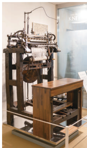
▲The world’s oldest sock knitting machine (devised by William Lee)
