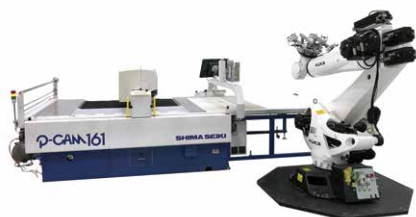
Automated pickup by connecting a P-CAM® and robot arm (exhibited at SAMPE Japan 2020)
