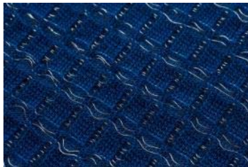
Inlay patterns limit typical stretch characteristics of knitwear
