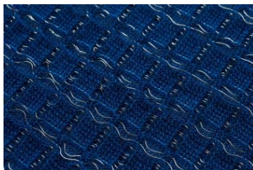
Inlay patterns knitting technology (involves inlaying a weft)
