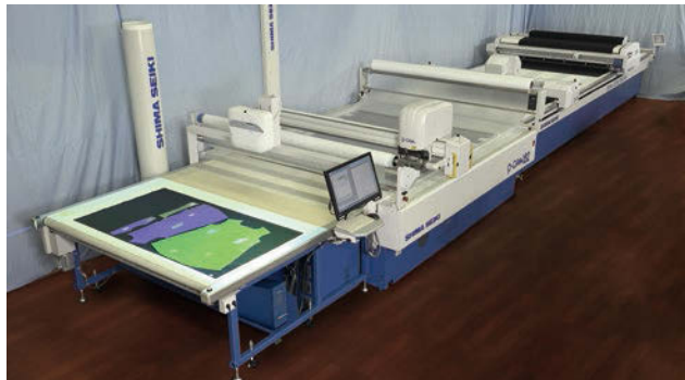
The “Total Cutting Solution,” which combines a computerized cutting machine and a computerized spreading machine
